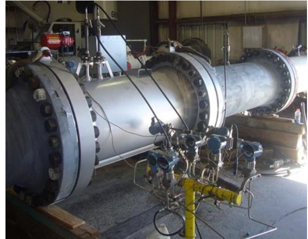
Fig 2. Dermaga / DP Diagnostics 24” Cone Meter Under Calibration at CEESI Iowa.
