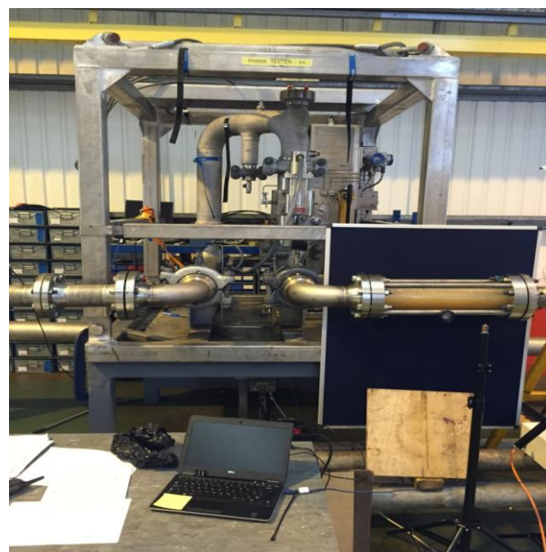
Figure 1: Intercomparison transfer standard and transparent pipe section used for flow visualization, as installed at NEL.
