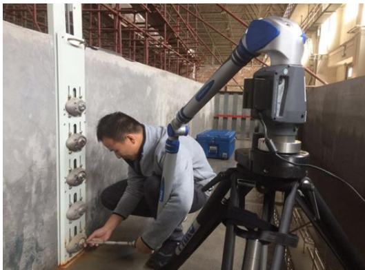
(a) photo of geometric measurement with FARO arm
