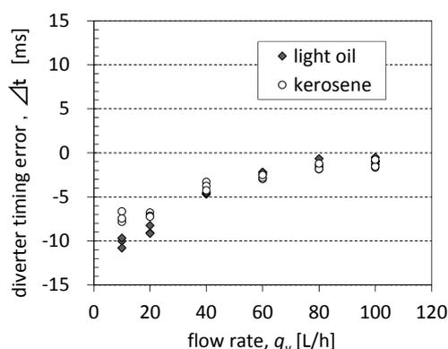
**Figure 3:** Diverter timing error of two diverters (after adjustment) using feeding nozzle with inner diameter of 4 mm.  $\blacklozenge$ : diverter for light oil,  $\circ$ : diverter for kerosene.
