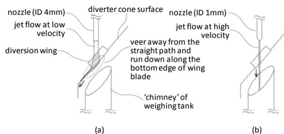
**Figure 4:** Jet flow behaviour along the surface of diversion wing. (a) Deviated flow path (flow rate 10 L/h, nozzle inner diameter 4 mm). (b) Straight flow path (flow rate 10 L/h, nozzle inner diameter 1 mm).
