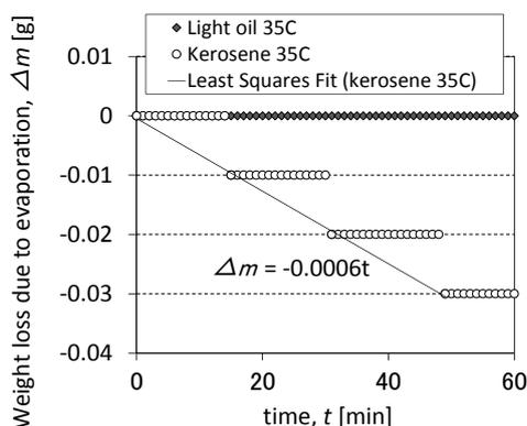
**Figure 5:** Weight loss due to evaporation over time (liquid temperature 35°C).
