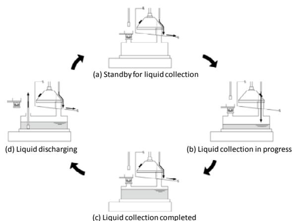
Figure 2: Operation sequence of gravimetric system.
