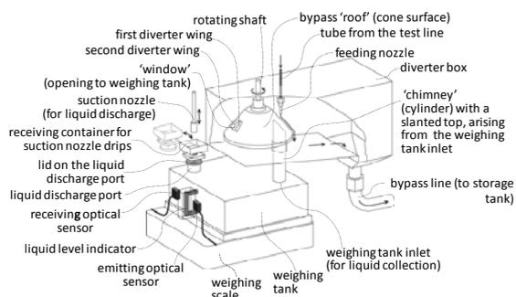
**Figure 1:** A new gravimetric system using conical rotating double-wing diverter (CRDWD); CRDWD at  $0^\circ/360^\circ$  position (diverter's window on the opposite side from feeding nozzle).
