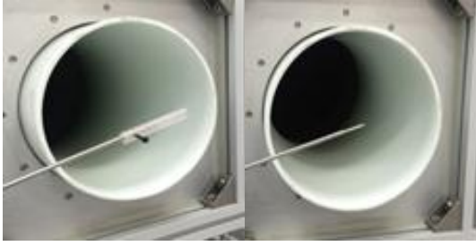
Figure 7 The probe calibrated in wind tunnel by LDV The air temperature in wind tunnel is 20.3^{\circ}\text{C} , and the static equation in theory is expressed by:
