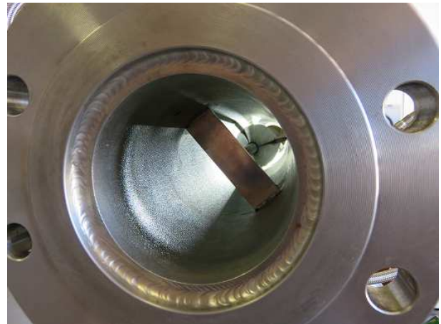
Fig 15. Looking Downstream in a 4" Vortex / Cone Mass Meter.
