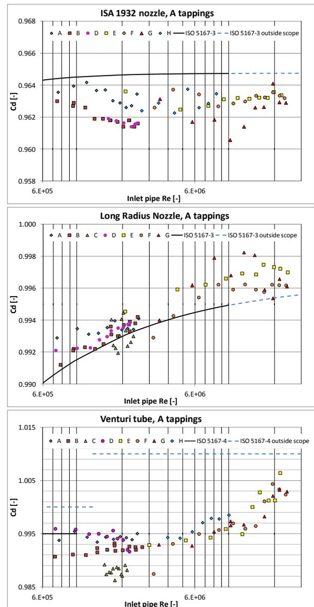
**Figure 3:** Calibration results for water, hot water and natural gas for the ISA 1932 nozzle (top), the long radius nozzle (middle) and the Venturi tube (bottom), all using the A tapplings. The  $C_d$  value is depicted versus the inlet  $Re_D$  number. The labs are represented by different colour dots. The solid black line is the literature value within the scope of the standard [2] [3], the dashed blue line is the range that is outside the scope.
