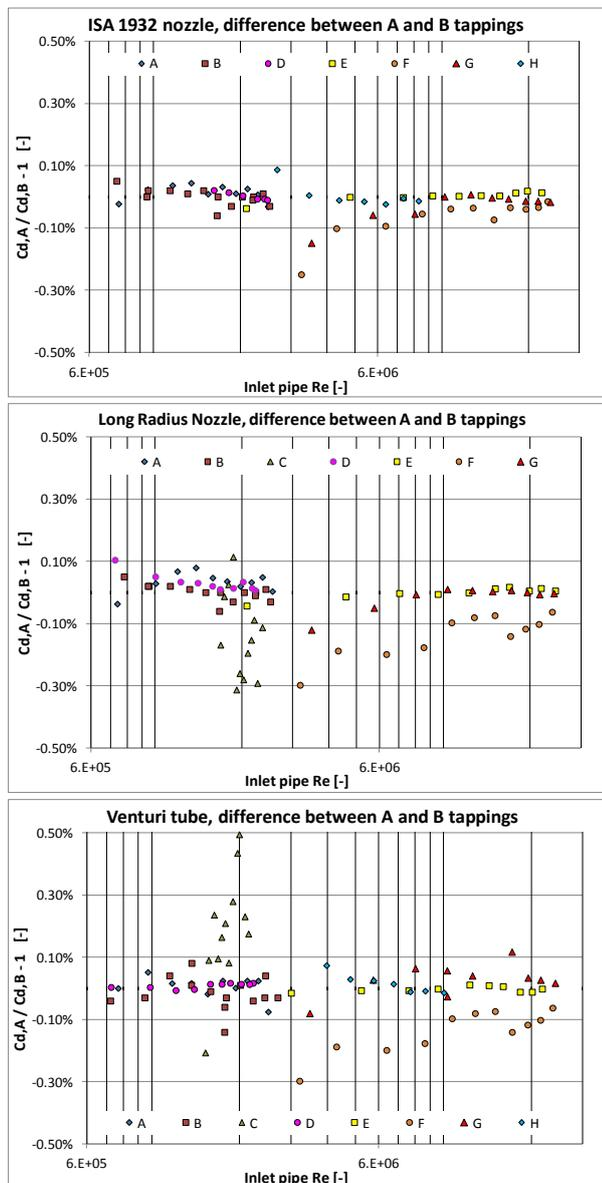
**Figure 2:** Percentual difference between  $C_d$  measured at A and B tapplings for an ISA 1932 nozzle (top), the long radius nozzle (middle) and the Venturi tube (bottom) as a function of the inlet  $Re_D$  number [-]. The labs are represented by different colour dots. Most results are between  $\pm 0.1\%$ . For the ISA nozzle the results of lab C were discarded.
