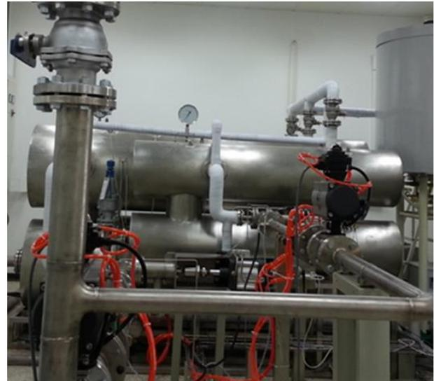
Fig.1: The high pressure pVTt gas flow standard facility
