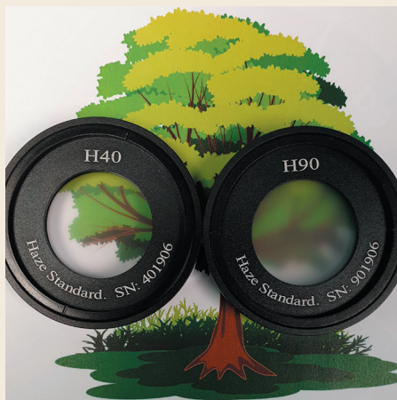
Figure 1. Photograph of two haze standards with different haze values – the left standard has a haze value of 40%, the standard on the right has a haze value of 90%.
