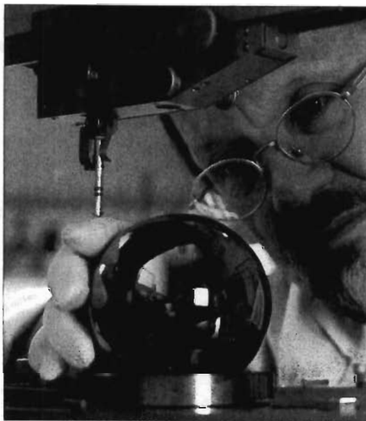
Achim Leistner setting up sphere for roundness measurement
