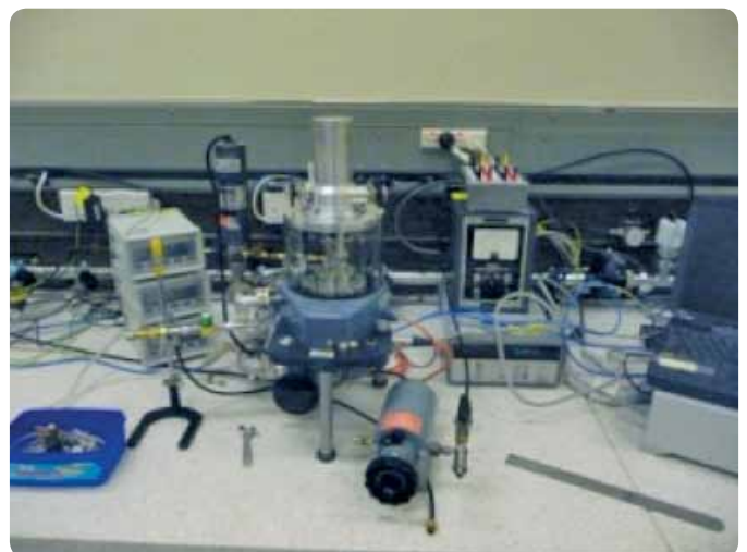
In the pressure lab, a Bell + Howell absolute pressure deadweight tester. It has a specially made manual mechanism (the aluminium assembly on the top) that allows masses to be lifted individually from the pneumatic piston without breaking the vacuum in the glass chamber.
